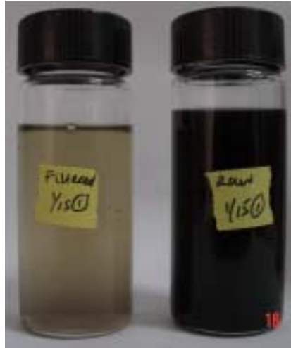
Figure 5-8: Left sample was incubated at 35°C for 24 hours and some black color can be seen at the bottom. MF results show 9 TC per 100ml. Right sample showed a positive H 2 S Test with TC exceeding 600 CFU per 100ml.
