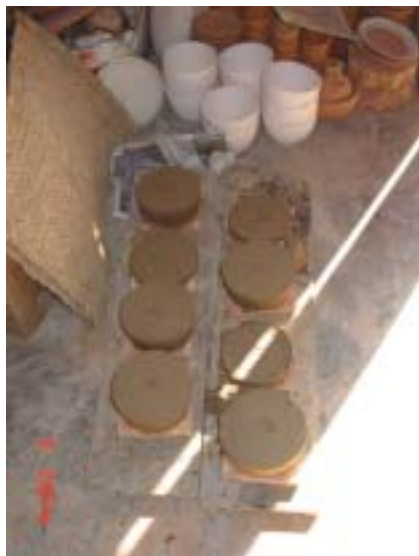
Figure 7-15: Mixtures allowed to dry for 5-7 days before firing.
