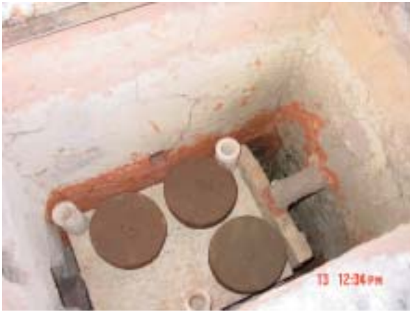
Figure 7-16: Dried mixtures are placed in the kiln and fired at a temperature of 1000-1070°C for 12 hours.
