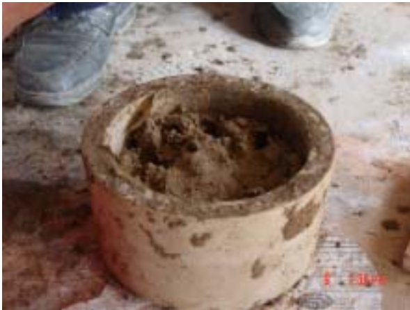
Figure 7-12: Mixture placed in a plaster mold made by Hari. The mold has an inner diameter of 6" and depth of 3".
