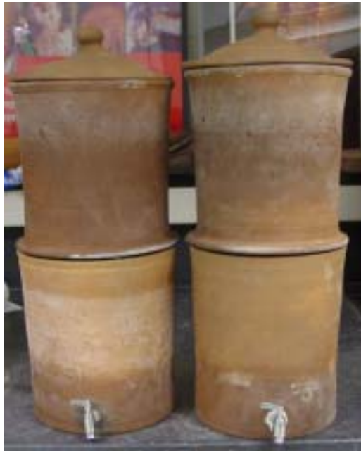
Figure 8-4: Two Thimi ceramic filters with ceramic filter disks of different compositions that are brought back to MIT.
