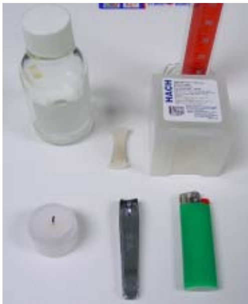
Figure 5-2: P/A test equipment and supplies for H_2S bacteria test. 100 ml sample bottle shown in picture.
