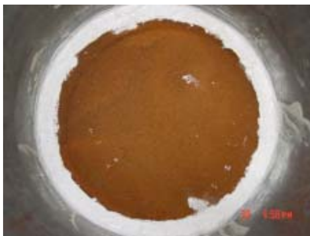
Figure 8-9: TERAFIL (MIT) showing the silicone added on top of the white cement after drying.
