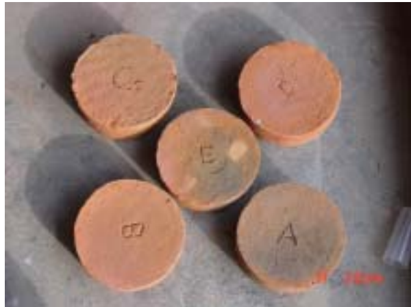
Figure 7-17: Filters after firing and ready to be affixed. Lighter color in filters after firing.
