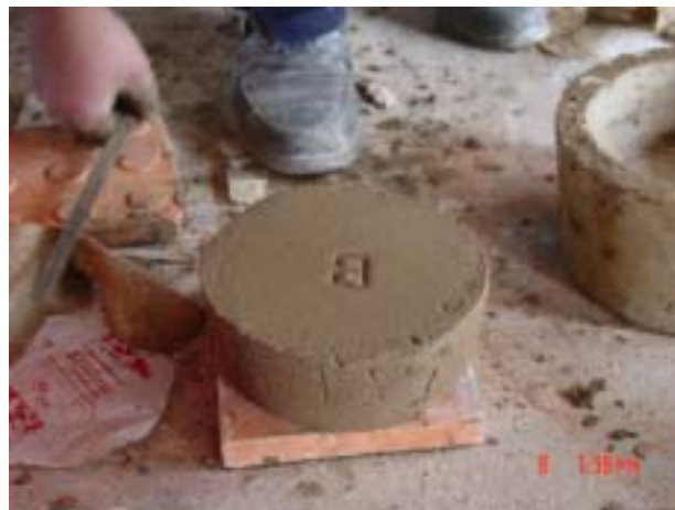
Figure 7-14: The mold is carefully inverted to remove the mixture and is labeled for easy identification.
