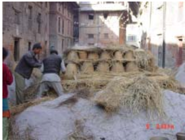
Figure 7-3: Pots ready to be fired in the traditional way are covered with hay and ash.
