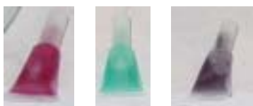
Figure 6-5: Plastic ampules are pre-packed with 2 ml of (from left to right) m-Endo, m-ColiBlue24 ® , m-FC media from Millipore.
