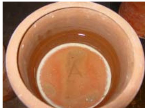
Figure 8-5: Top view of the upper container showing the ceramic filter disk A.
