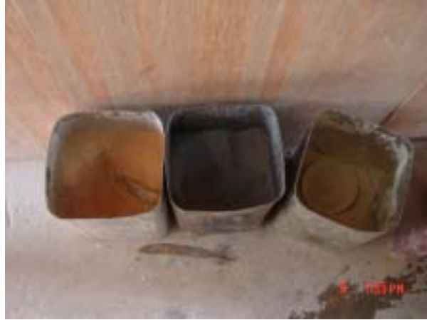
Figure 7-9: Three basic raw materials (from left to right) – Red pottery clay, rice husk ash, and sawdust.
