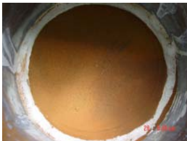
Figure 8-8: TERAFIL (MIT) showing the original white cement used to bond the ceramic filter to the metal container.
